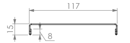
REINFORCING CHANNEL I DETAIL
