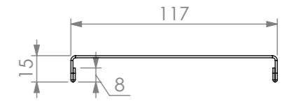
REINFORCING CHANNEL I DETAIL
