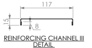
REINFORCING CHANNEL III DETAIL
