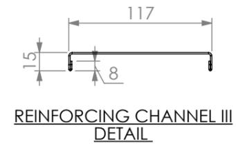
REINFORCING CHANNEL III DETAIL
