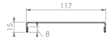
REINFORCING CHANNEL III DETAIL
