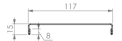
REINFORCING CHANNEL I DETAIL
